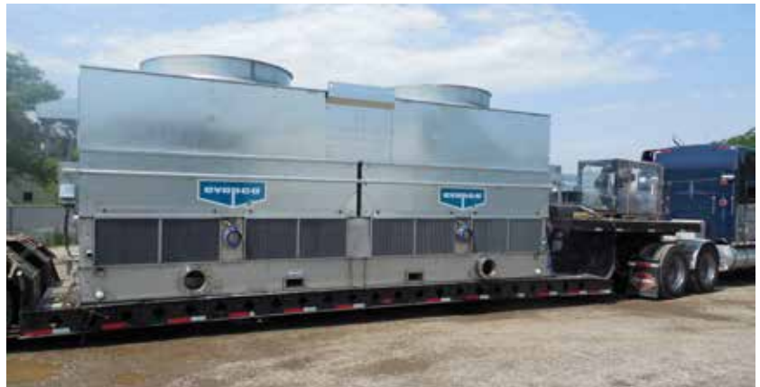
500 Ton Cooling Tower
